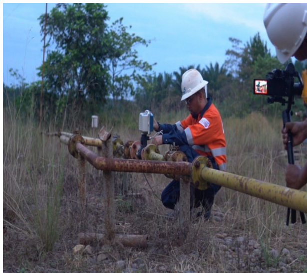
Regular monitoring to observe the gas rate readings and other relevant parameters during the dewatering process at MU-005TW
