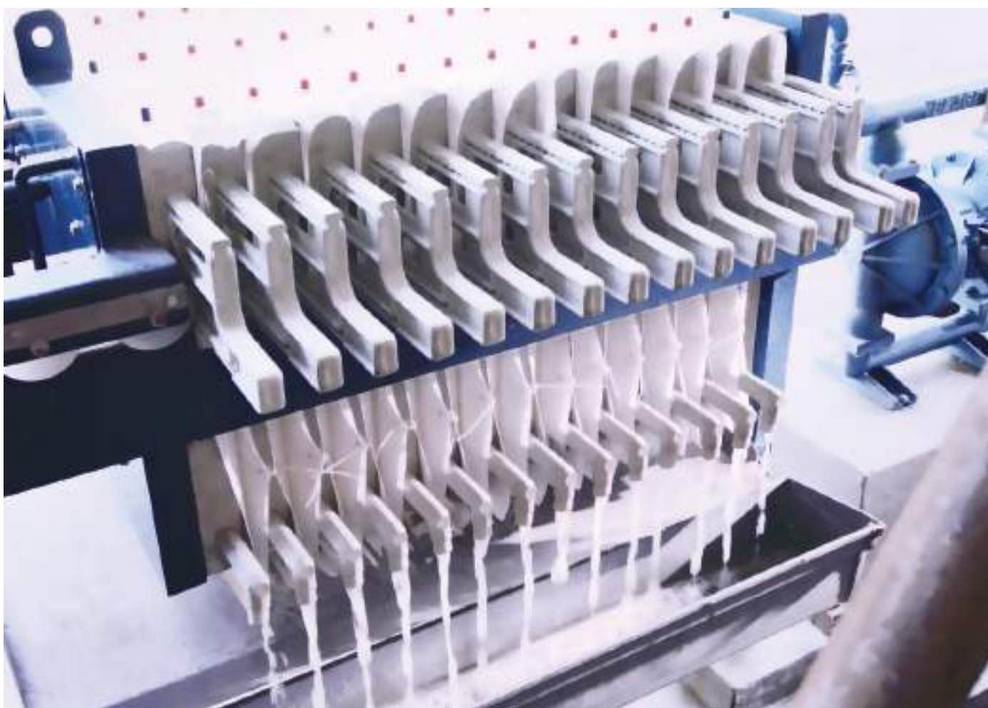
Our filter press process to remove excessive water from solid waste
