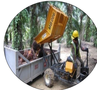
SD2 System: Two-tier bin system with mechanical buffalo
