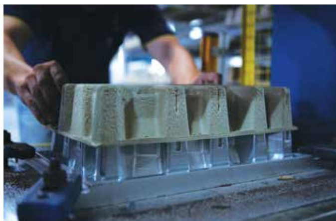
Above and below: CBB Senai leads the way in producing moulded pulp casings in Malaysia, utilising 100% post-industrial raw materials.
