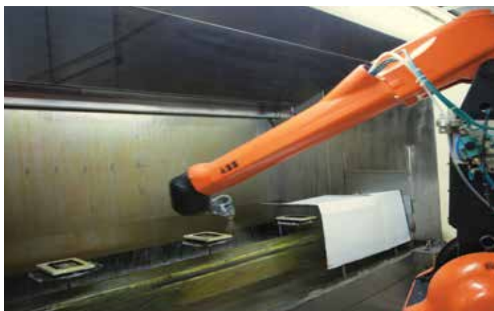
Fully automated spray painting process at CPI's plastic injection moulding plant.
