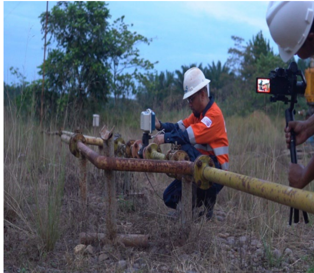
Regular monitoring to observe the gas rate readings and other relevant parameters during the dewatering process at MU-005TW
