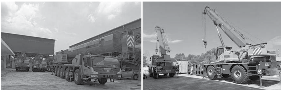
Left: Truck-mounted crane; Right: Rough terrain crane
