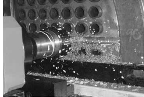
Tube sheet groove milling
