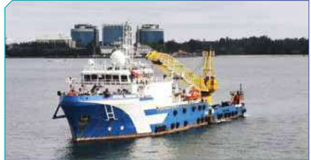
M.V. KEYFIELD COMMANDER DP2 Accommodation Work Boat
