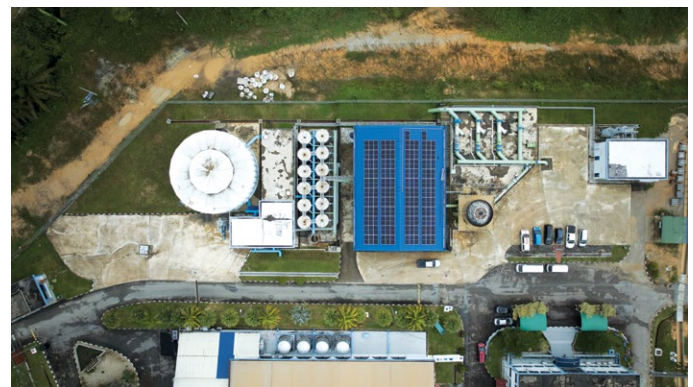
▲ Ranhill's 54 kWp Solar PV System at the 20 MLD Sultan Iskandar WTP Extension Project
