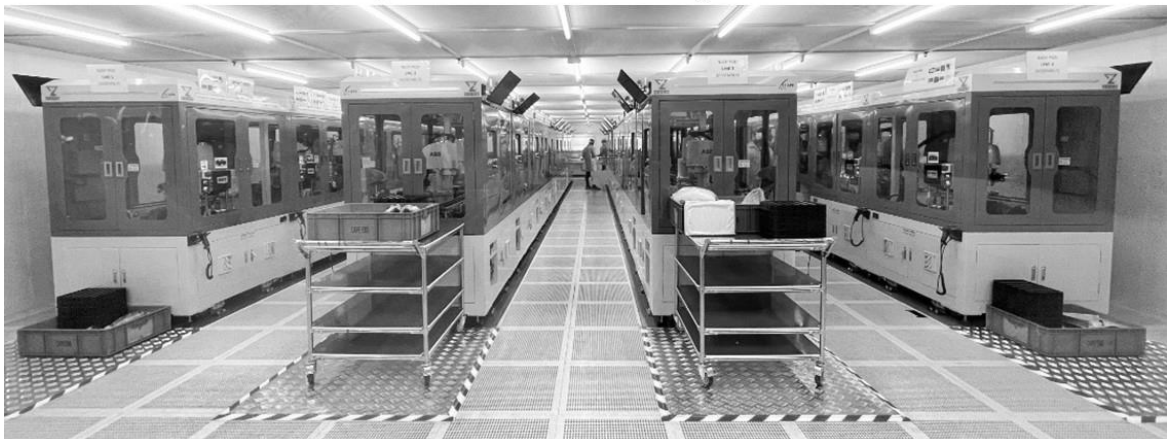
Automated production lines for electronic cigarettes in cleanroom
