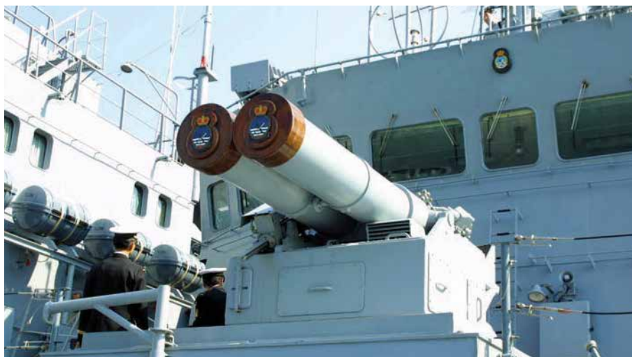
Bofors 375mm Anti-Submarine Rocket Launcher maintained by BHIC Bofors Asia Sdn Bhd, a JV Company Bofors Sweden onboard an RMN ship. BHIC Group provides comprehensive MRO services to Malaysian Armed Forces assets
