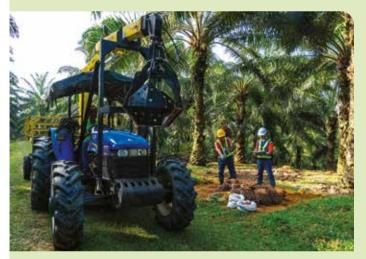
Mechanising our operations - loading of fresh fruit bunches (FFB) using crane and grabber.
