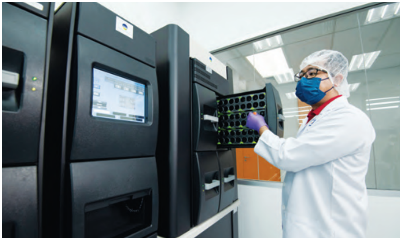
Finished product sterility test
