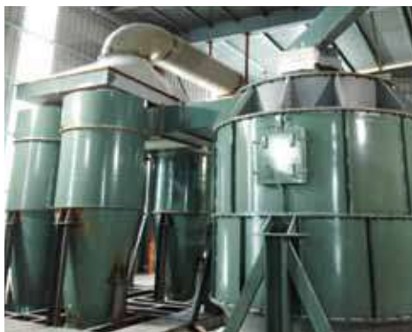
Picture: Cyclone and Classifier installed at Green Cement's Grinding plant located in Kota Tinggi, Johor
