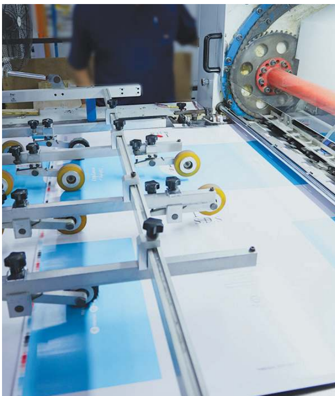
Laminating the outer layer of offset carton boxes with printed sheets for finer and more vibrant printing quality.
