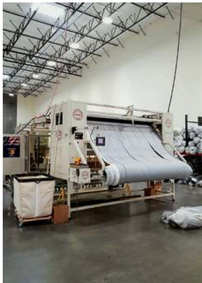
Quilting machine for mattress border panels.
