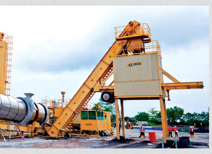
In FY 2016, two mobile premix plants with a capacity of 150 MT and 100 MT per hour respectively were purchased. These mobile premix plants will be set up at Limbang and Samalaju this year to meet increasing demand within these regions. An existing 40 MT per hour mobile premix plant at Limbang will be mobilised on a project basis. The Division plans to further expand its premix capacity by purchasing two additional mobile batched premix plants for the Pan Borneo Highway project.
