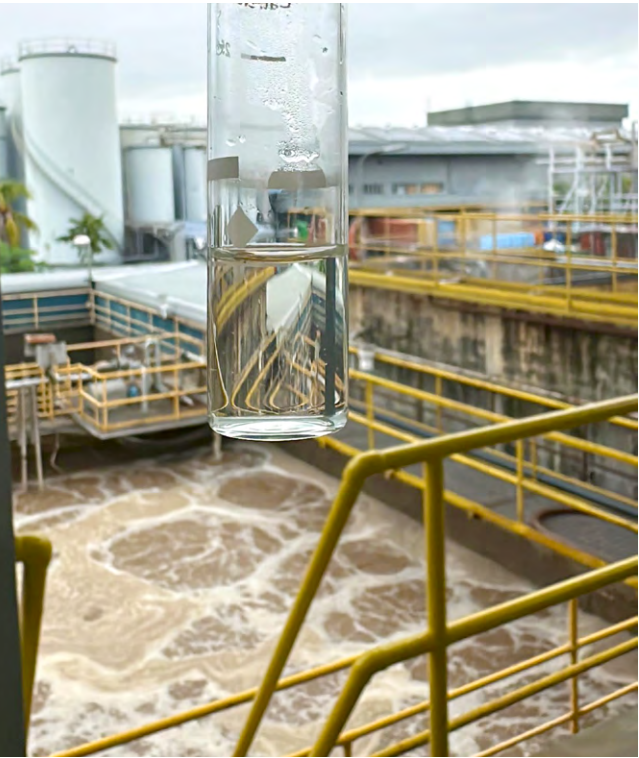
>> Effluent clarity post-treatment – a clear water sample from SD Guthrie International Langat, showcasing the effectiveness of the Oil Recovery System in treating CPO washing effluent whilst recovering technical-grade oil before discharge.
