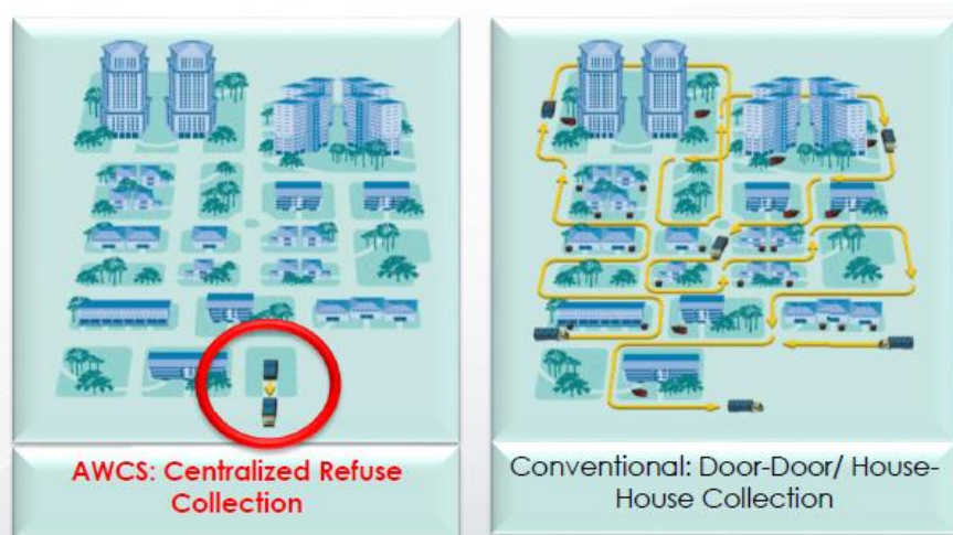
Figure 1: How STREAM differs from conventional waste collection
