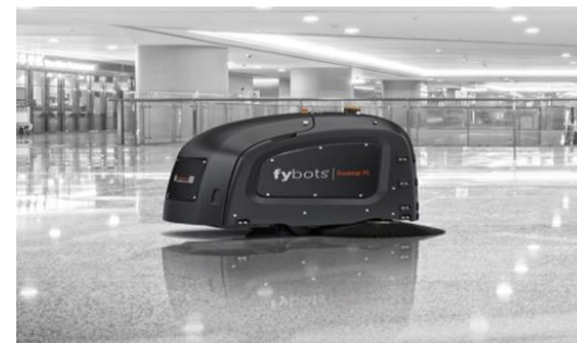
Mechanisation of cleaning processes via an autonomous scrubber
